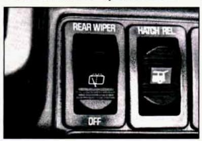
You control your rear window wiper/washer from a switch on your instrument panel, on the driver's side of your steering column.
